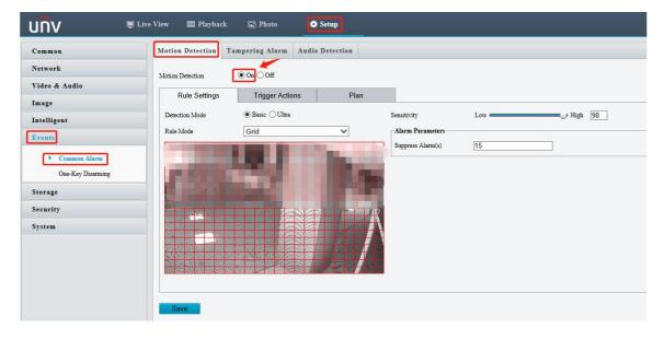
**Step 2.1** Create an alarm task on the Unicorn's web interface under **Alarm Configuration**.
